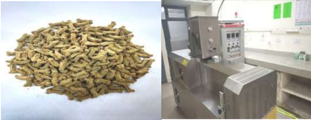
Plate 1: Extruded dog food and twin screw extruder
