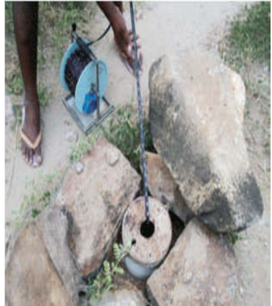
Water level measurement in borewell by using a water level indicator
