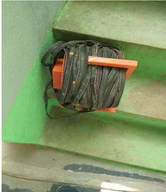
Water level measurement in borewell by using a water level indicator
