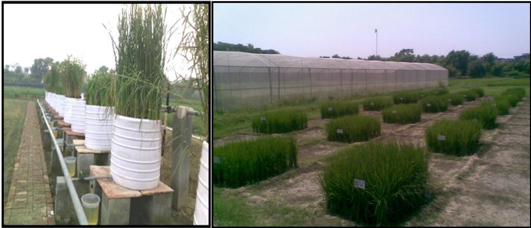
Figures 3.3: (a) Experimental wastewater treatment system based on vertical sub-surface flow (VSSF) constructed wetland technology (b) Experimental micro-plots
