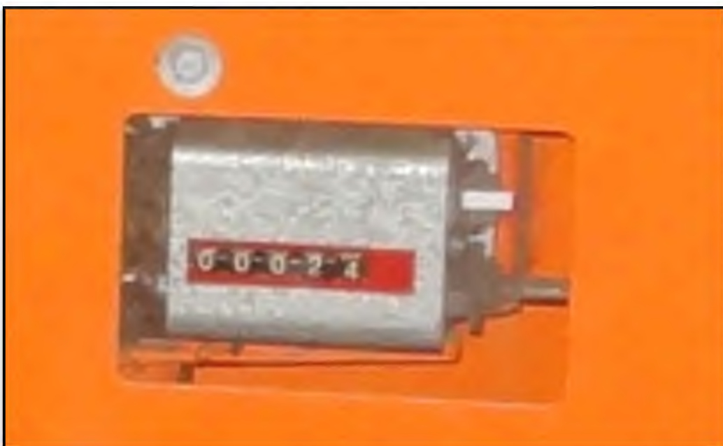
Plate 3.8 View of bale counter unit in the tractor-drawn round straw baler
