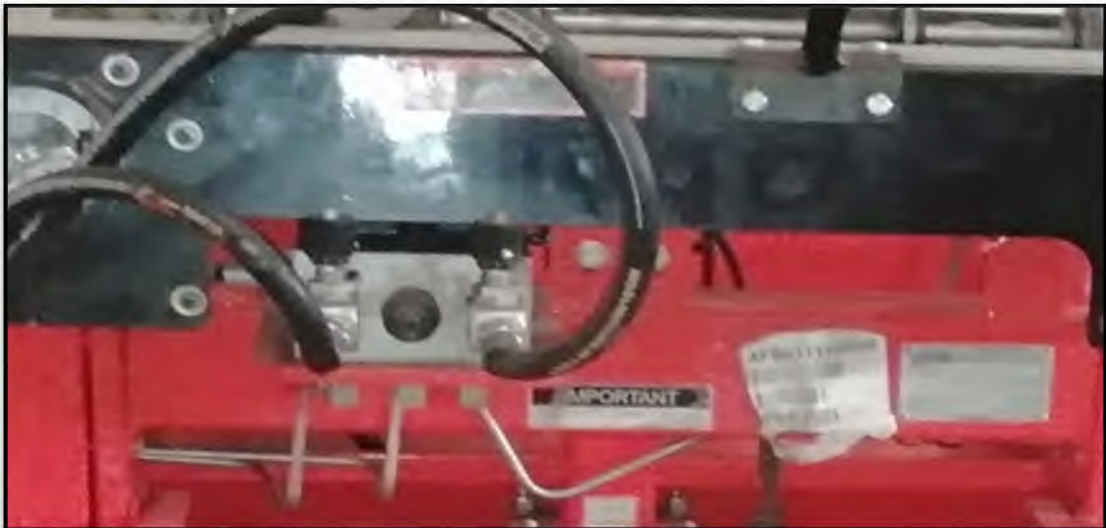
Plate 3.6 View of hydraulic valves in the tractor-drawn round straw baler
