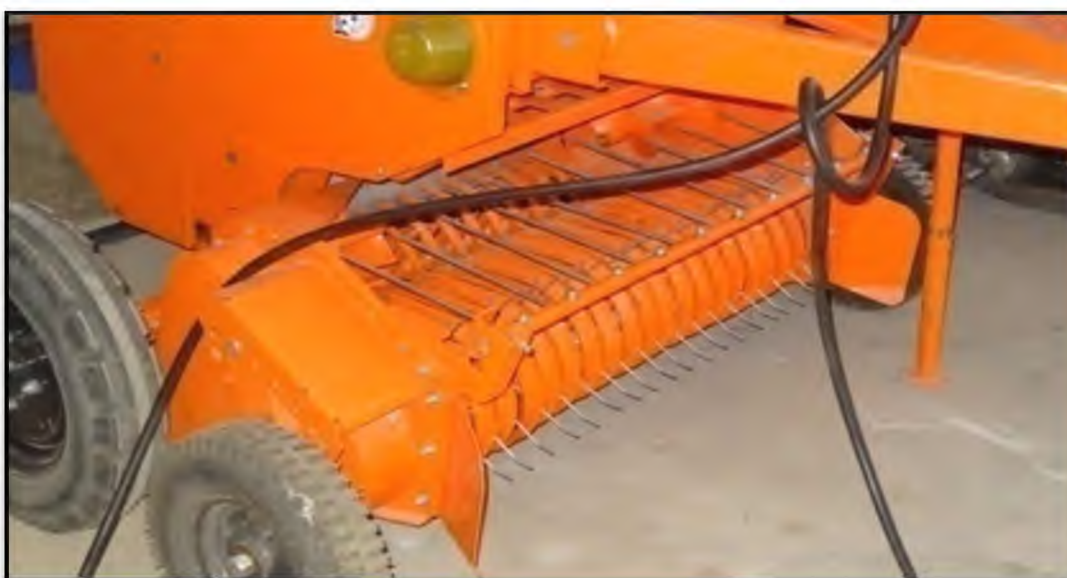
Plate 3.2 View of pick up unit of the tractor-drawn round straw baler
