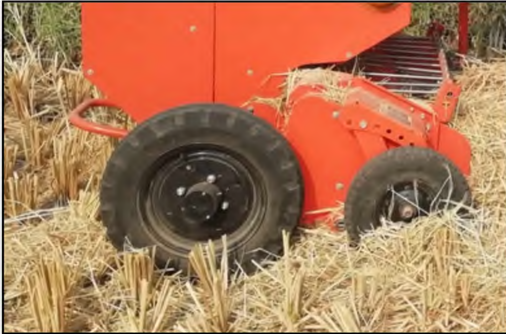
Plate 3.7 View of the floating tire of the tractor-drawn round straw baler
