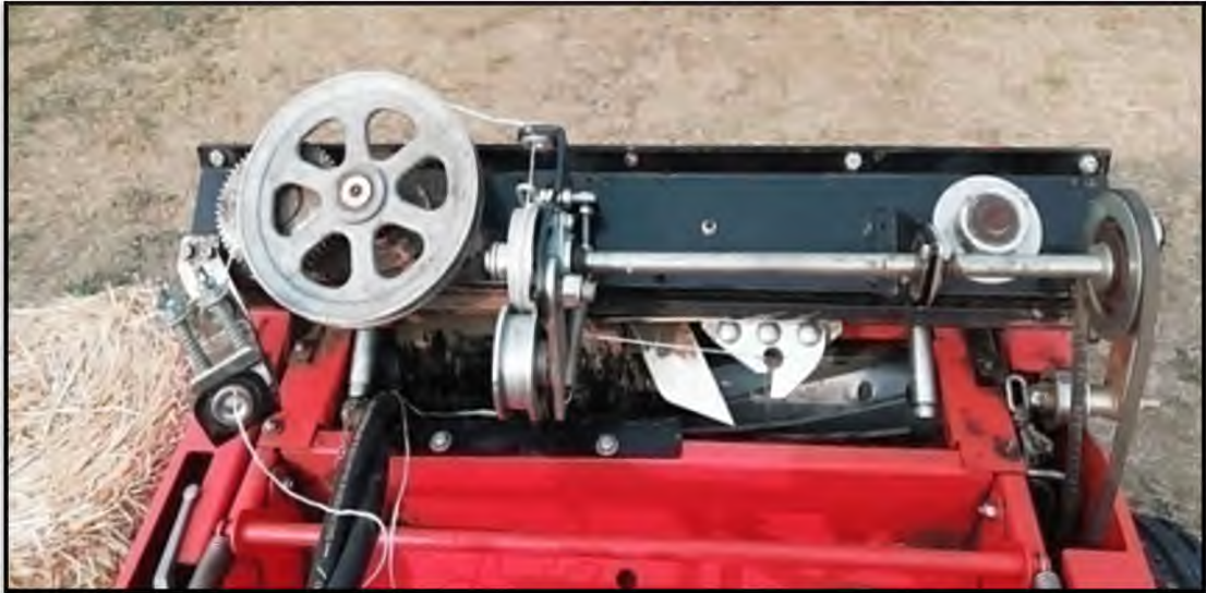
Plate 3.5 View of a binding unit of the tractor-drawn round straw baler
