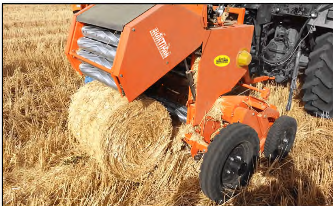
Plate 3.3 View of bale chamber & aluminium roller of the tractor-drawn round straw baler
