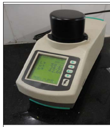
Plate.3.8. Hunter Lab colorimeter (Model: ColorFlex, Hunter Lab, USA)
