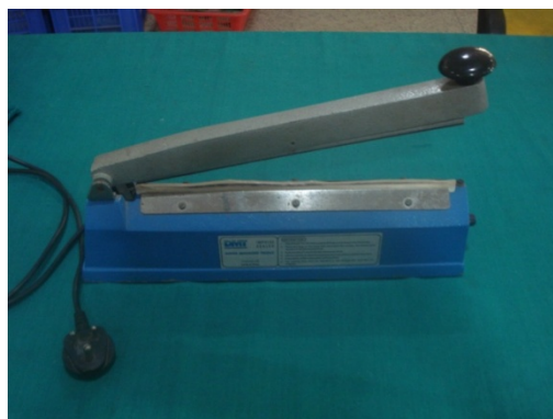
Plate.3.2. Hand operated sealing machine(DMT, Impulse sealer, Divya machine tools)
