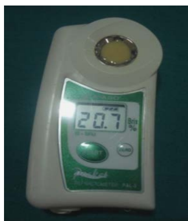
Plate.3.5. Brix Meter (Pocket Refractometer, Atago)
