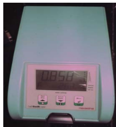
Plate.3.4. Water Activity Meter(Make: Labswift-a w Model: Novasina AG)
