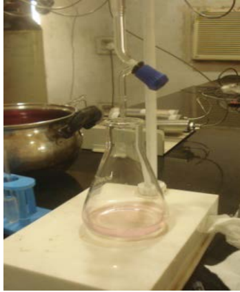
Plate.3.7. Acidity measurement (Titration method)
