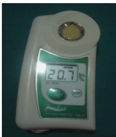
Plate.3.5. Brix Meter (Pocket Refractometer, Atago)
