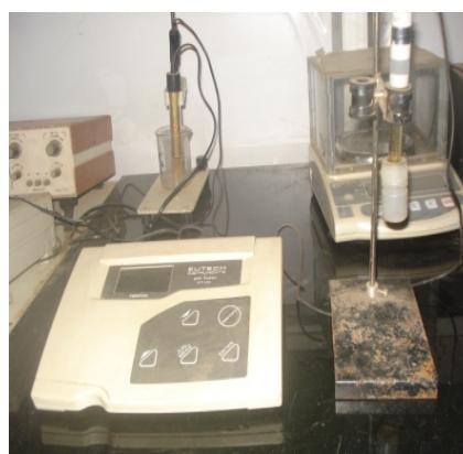
Plate.3.6. Digital pH meter (EUTECH Instruments)
