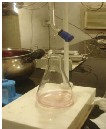
Plate.3.7. Acidity measurement (Titration method)
