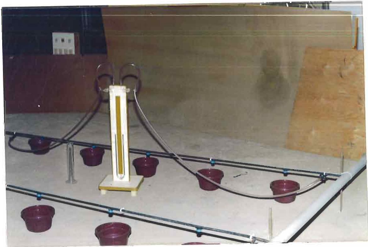
Segmental hydraulic gradient assessment using 'U' tube manometer
