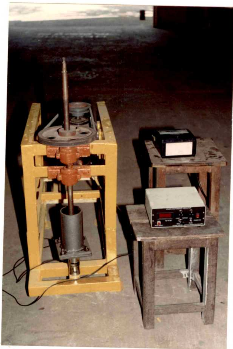
Plate 1 Experimental set up for the determination of the kinetic co-efficient of friction
