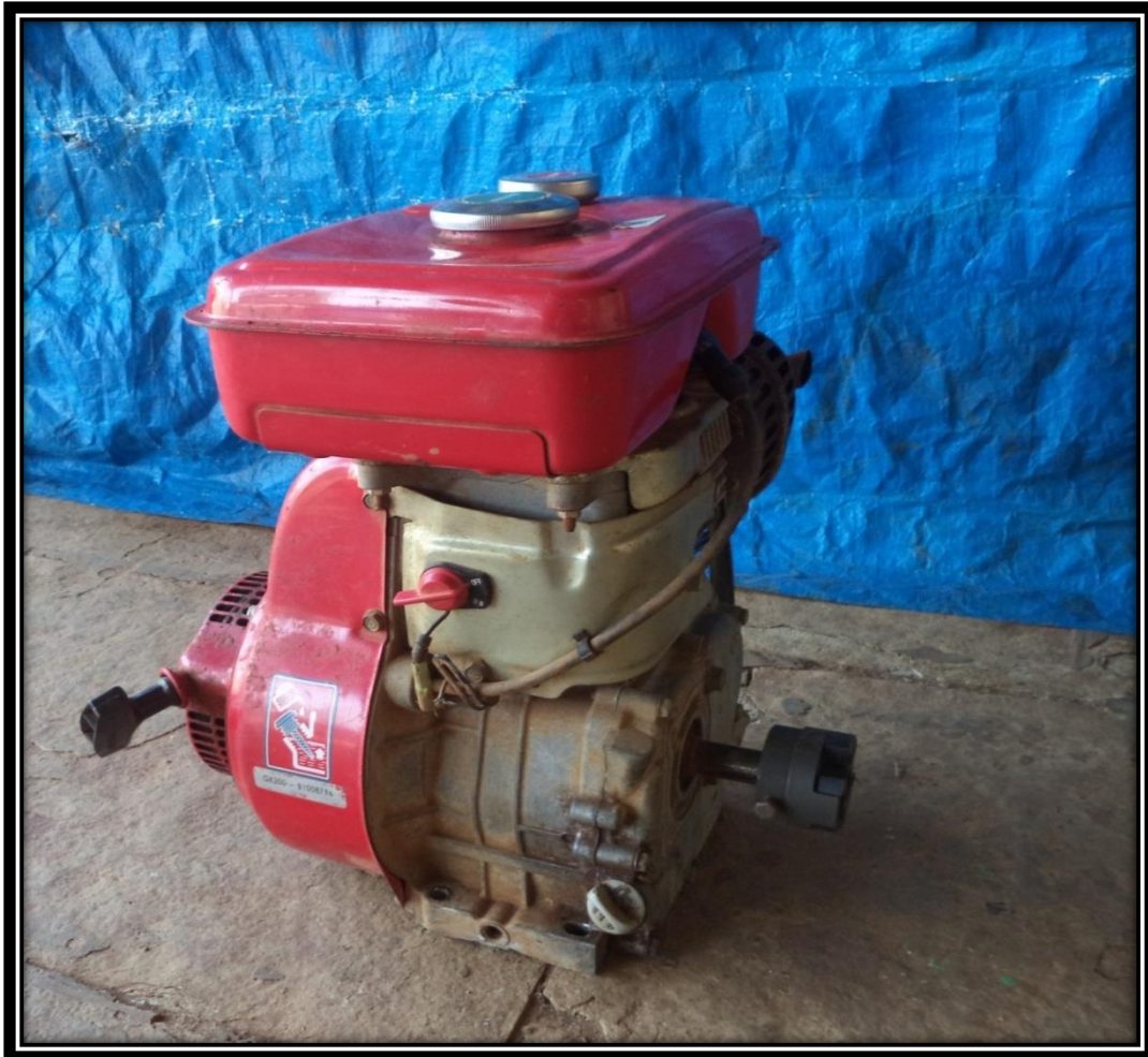
Plate 4.1 Honda engine (GK 200) used for power transmission
