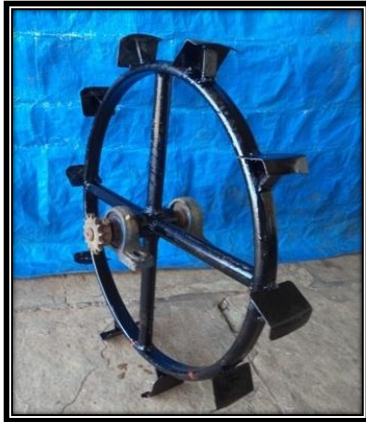
Plate 4.7 Drive wheel for forward motion of paddy transplanter
