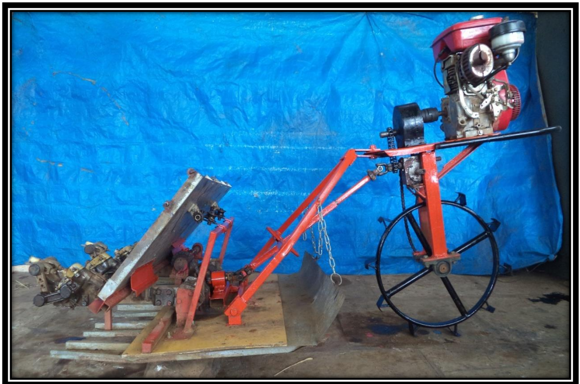
Plate 4.8 Developed self propelled paddy transplanter
