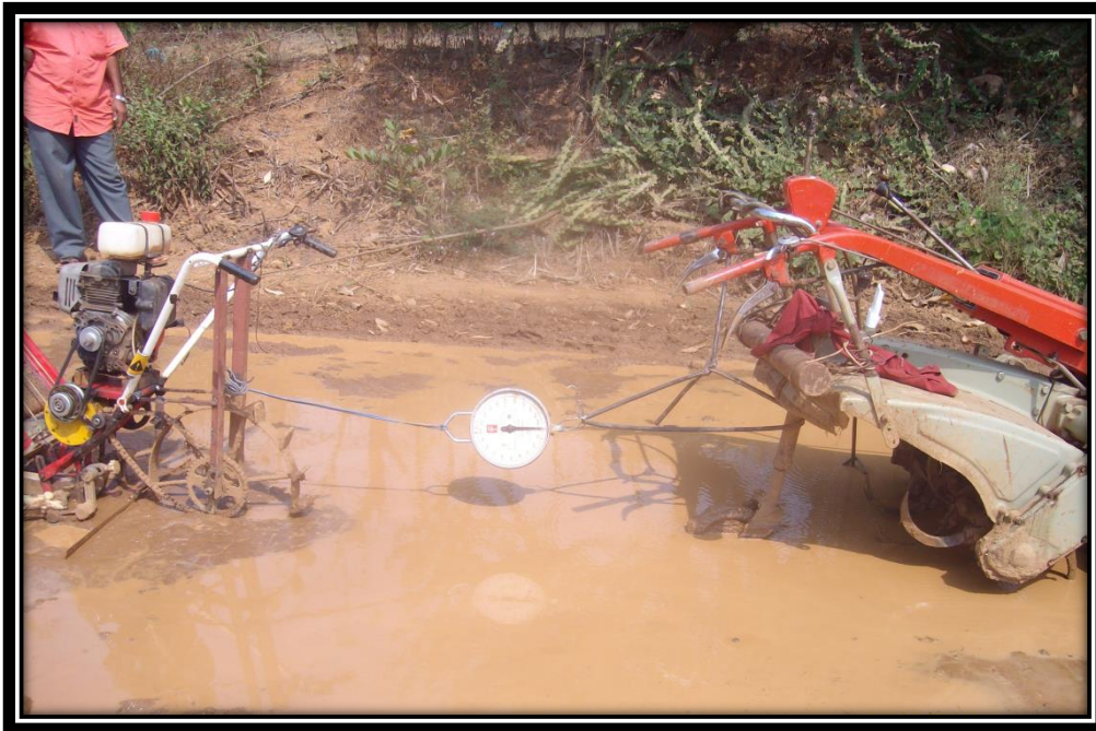
Plate 8.1 Measurement of drawbar rolling resistance for two row transplanter
