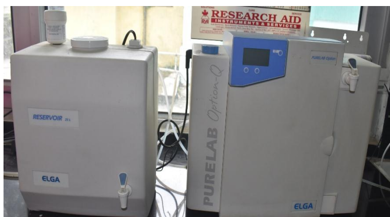
Ultrapure water purification system
