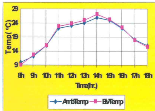
Fig. 12. Diurnal variation of temperature within the OTC
