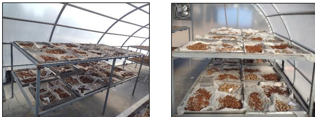
Plate 3.10 Solar tunnel drying of turmeric
