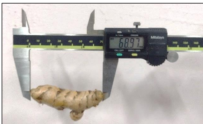
Plate 3.4 Measurement of dimensions of turmeric rhizomes using Vernier caliper
