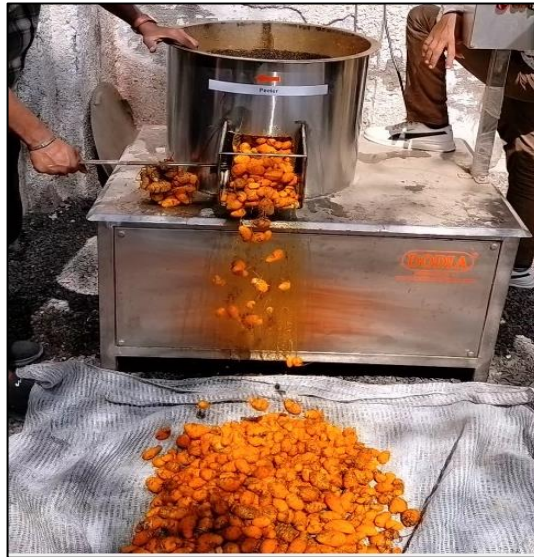
Plate 3.7 Peeling of turmeric rhizomes was done by using a mechanical peeler
