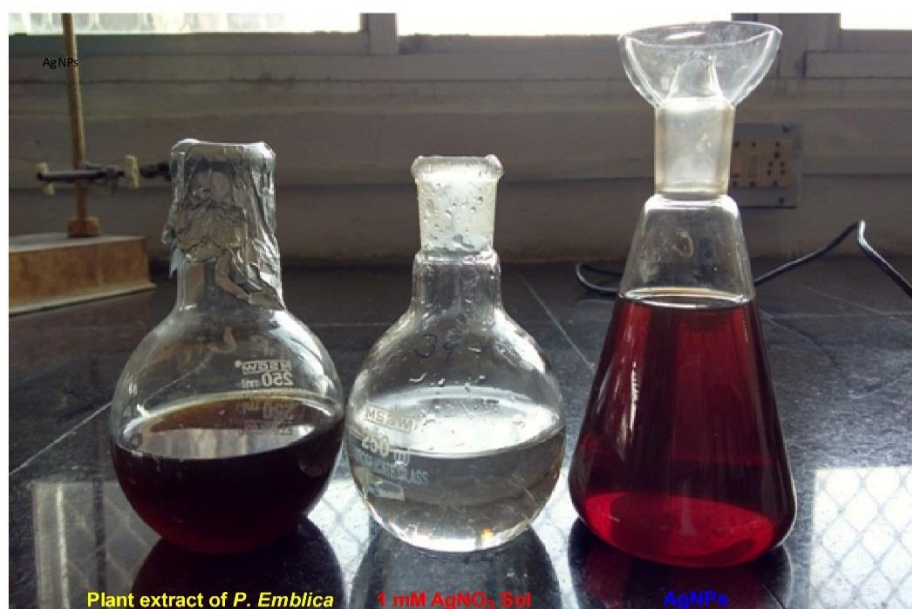
Figure 4.2 Biosynthesis of silver nanoparticles of P.emblica aqueous extract
