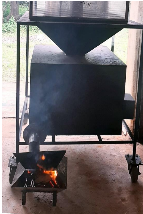
Plate 3.10: Burning of briquettes in biomass fired furnace
