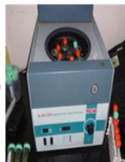
Centrifuge for 3 min at 2500-300 rpm to separate organic layer
