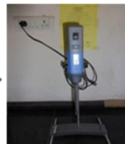
Homogenization at 14000 rpm for 2-3min with silent crusher (low volume Homogenizer)
