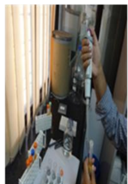
Take 8 ml extract into 15 ml tube with 0.4 g PSA and 1.2 g anhydrous MgSO 4
