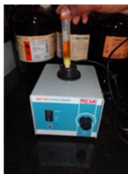
Add 9 g anhydrous sodium sulphate to remove moisture and mix with vortex
