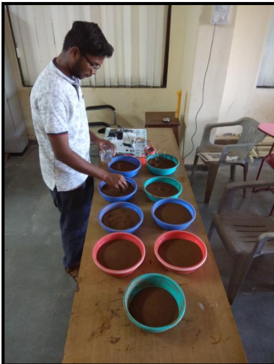
Plate 3.16 Addition of known amount of water to the oven dried soil sample and mixing it uniformly
