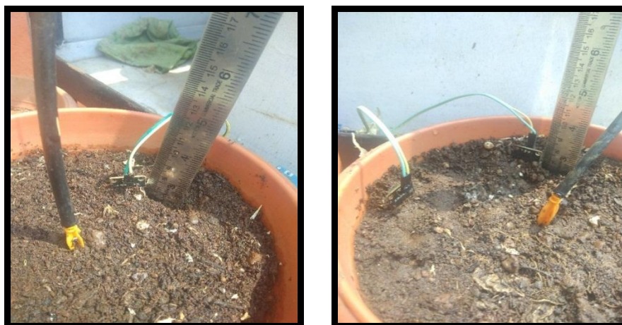
Plate 4.2 Soil Moisture Sensors installed in the pot
