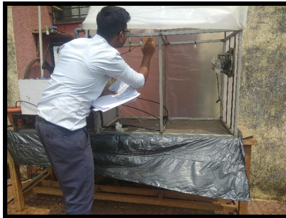
Plate 4.6 Recording the Readings of Masons Hygrometer
