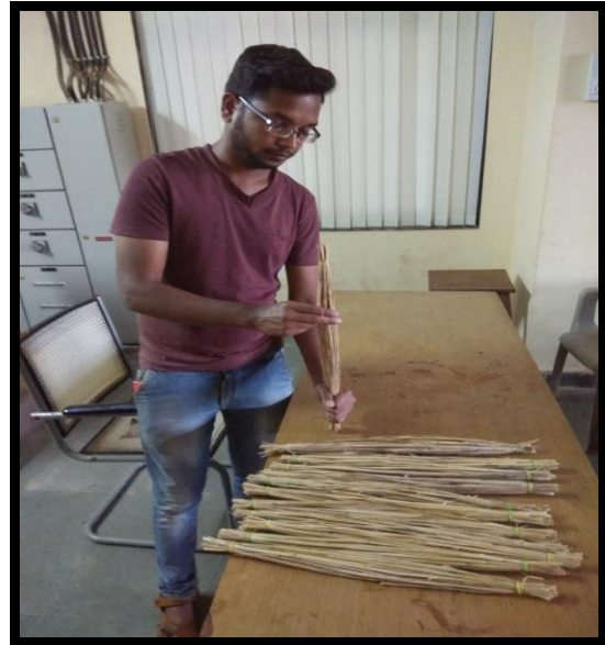
Plate 3.22 Preparation of Cooling Pad
