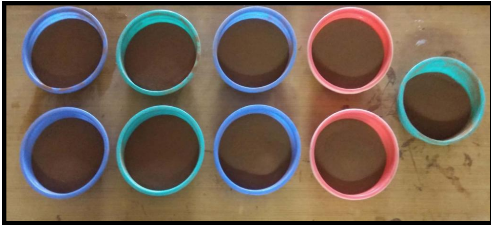
Plate 3.15 Nine sets of one kilogram oven dried soil samples for calibration of Soil Moisture Sensor
