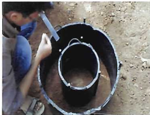
Plate 3.2. Marking of water level in the outer and inner ring
