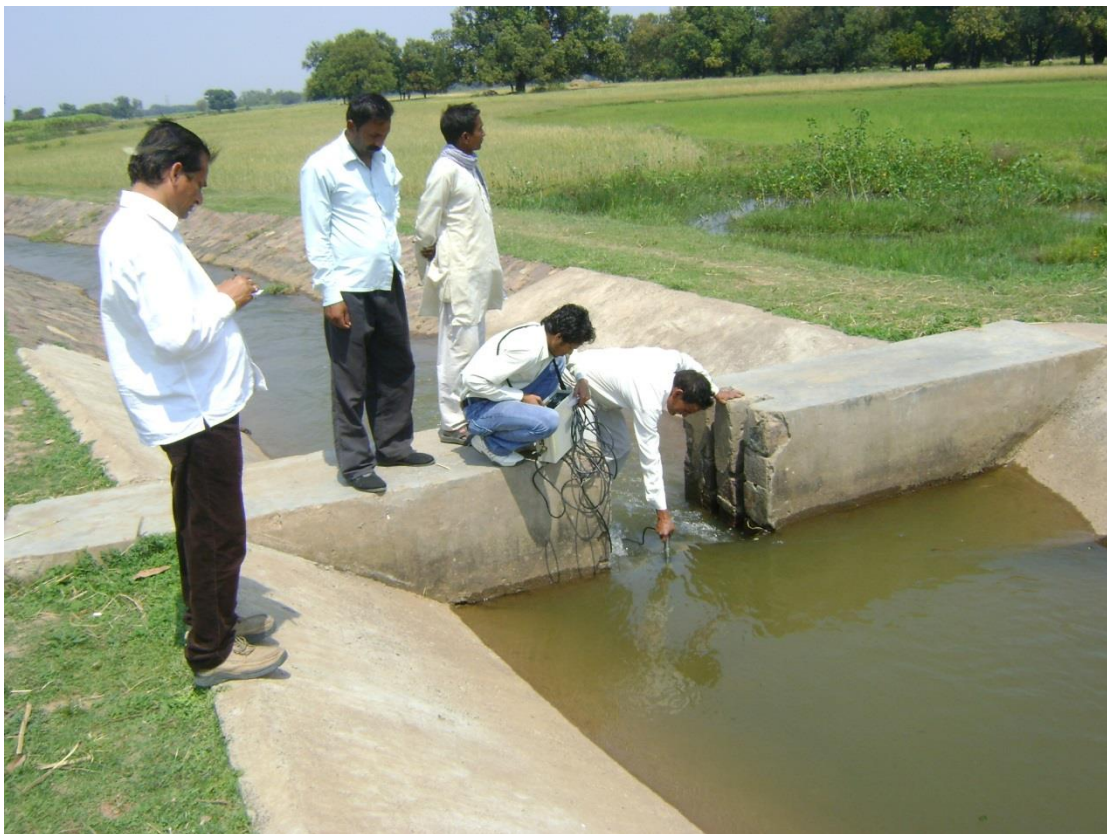
Plate 3.3 Measurement of canal water flow velocity in head reach.
