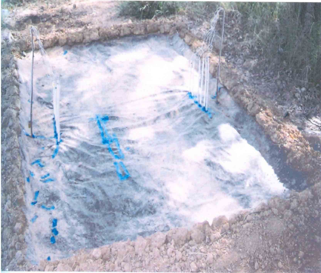
Plate 1: Experimental set up for in situ hydraulic conductivity determination
