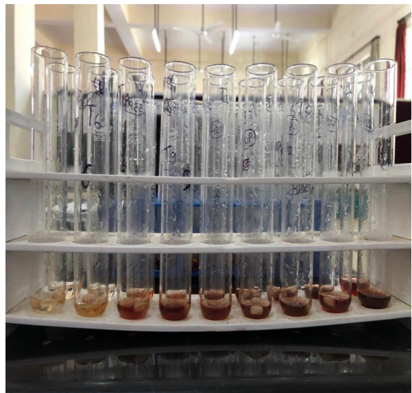
Colour gradient developed on the seed coat due to peroxidase activity
