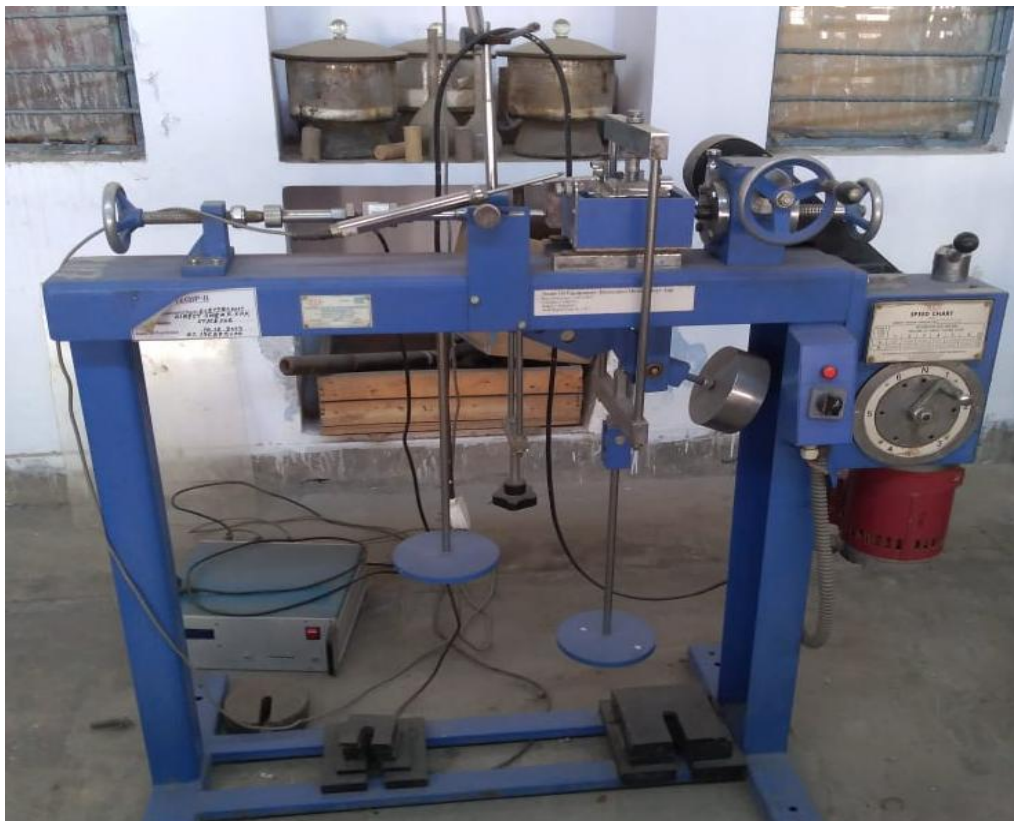
Fig. 3.6 Standard Direct Shear Test Equipment
