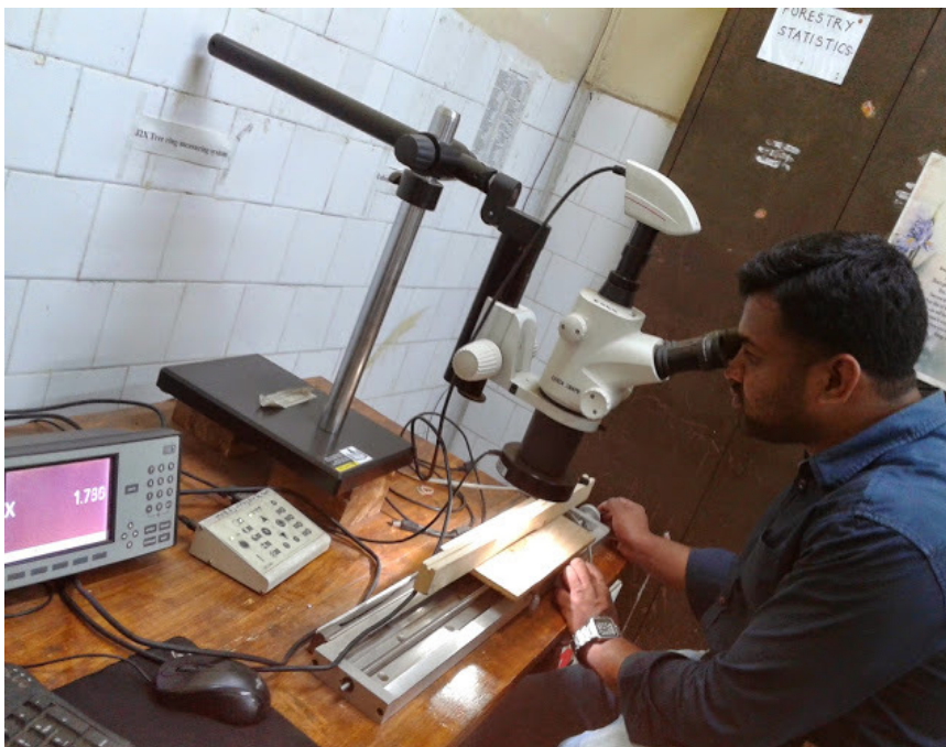
Plate 5: Measuring of Wood Growth Rings
