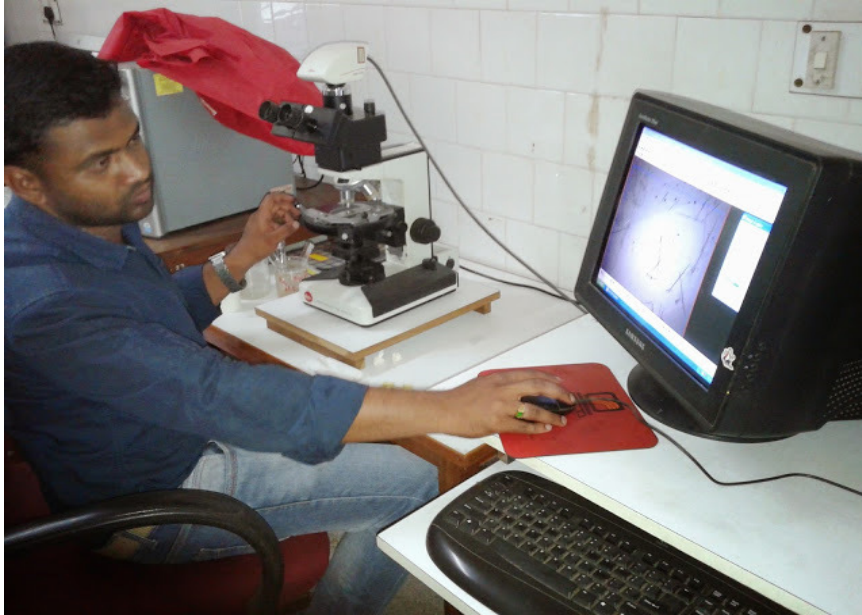
Plate 6: Measuring of wood fibre length
