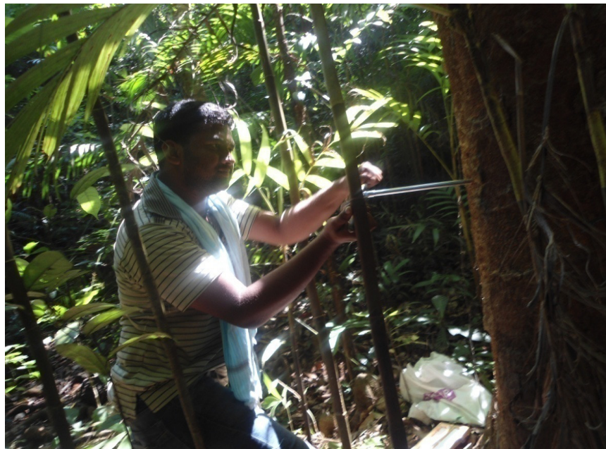
Plate 4: Collection of wood core sample
