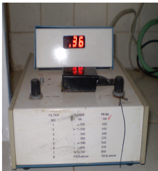
Plate 3.8: Colorimeter to Read the Green to Dark Green Color at 630nm for the Estimation of Carbohydrates
