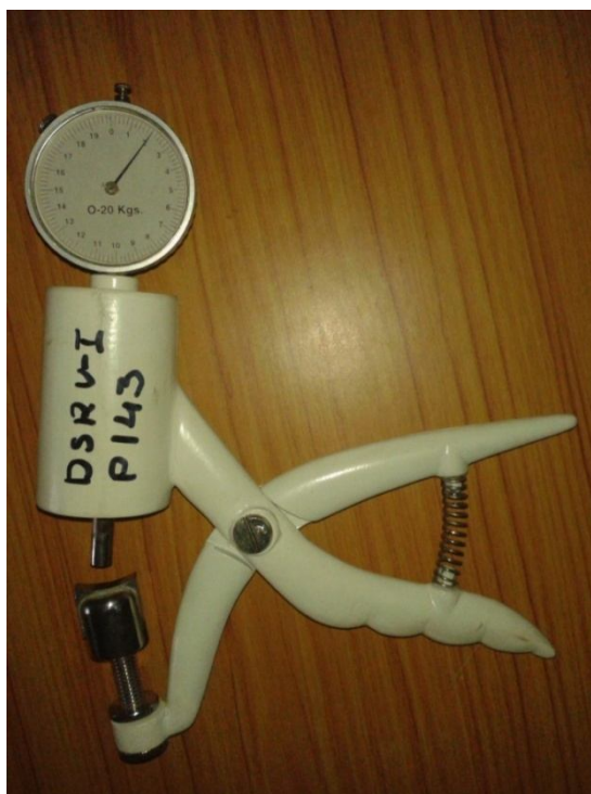
Plate 3.9: Measurement of hardness of chips using tablet tester
