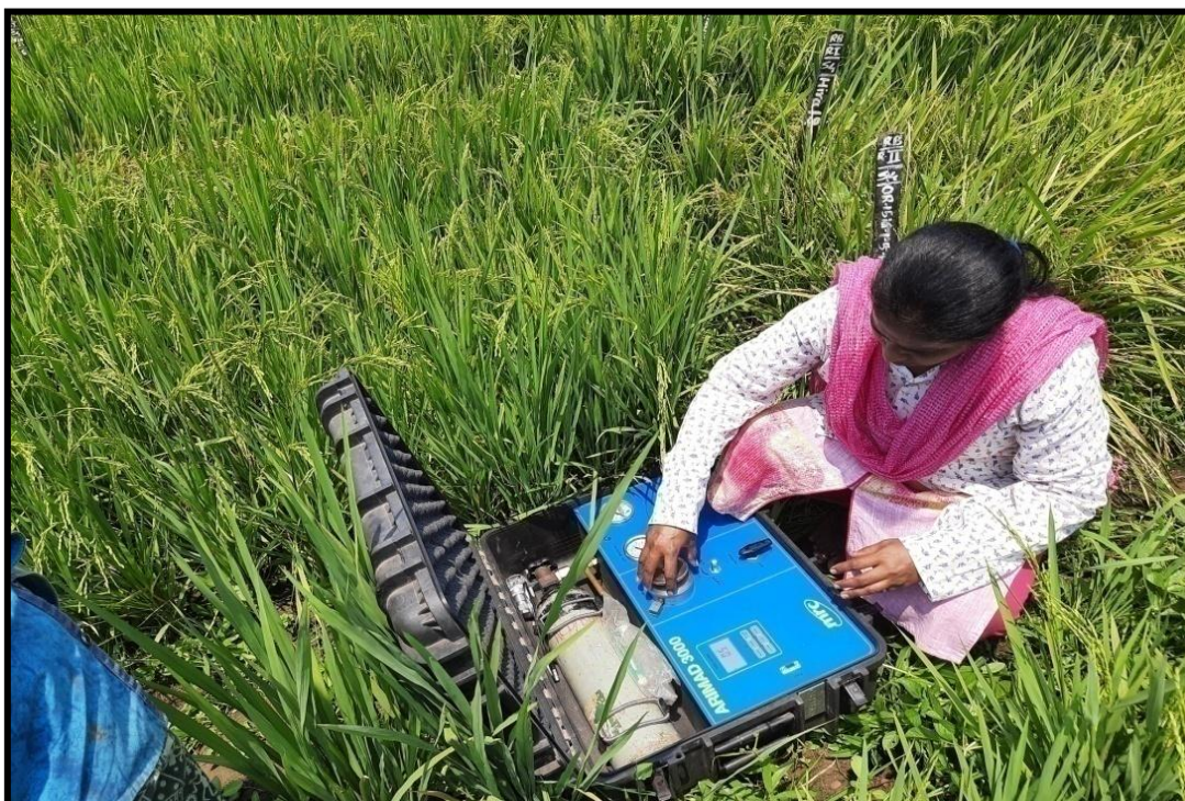
Plate IV : Measurement of leaf observations by portable pressure chamber (Arimad-3000) in experimental field
