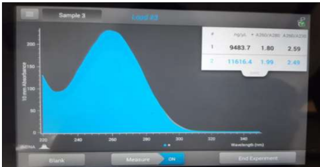
Figure 4.2: quantity analysis: -OD260/280 ratio-1.99-2.04 Concentration of 9000ng-12,000ng/μl
