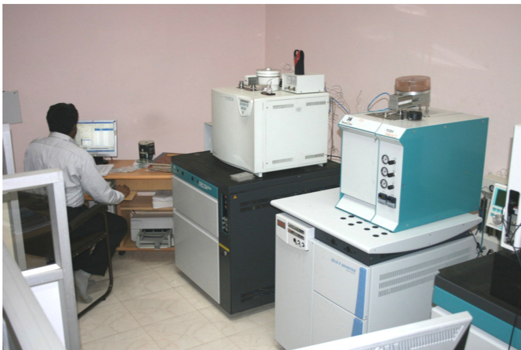
Plate 5. Isotope Ratio Mass Spectrometer (IRMS) facility for measuring stable isotope discrimination in plants
