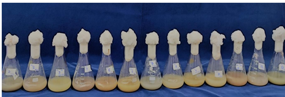
Plate 4.1: PBD 13 experiments by using Erlenmeyer flask containing medium components as per matrix Fusarium pallidorozeum
