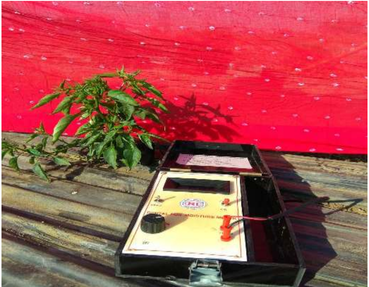
PLATE -2 Taking reading of soil moisture by digital soil moisture meter
