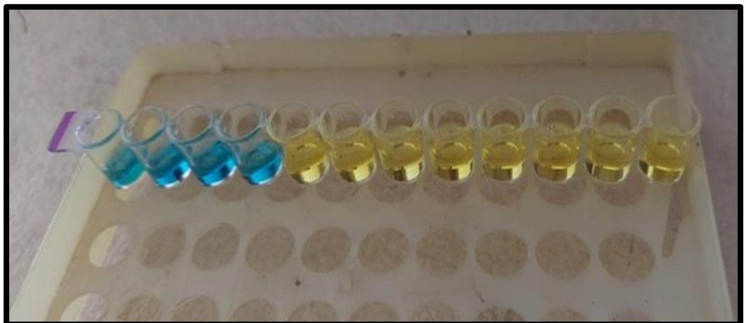
Plate 4. Color development on the addition of stop solution
