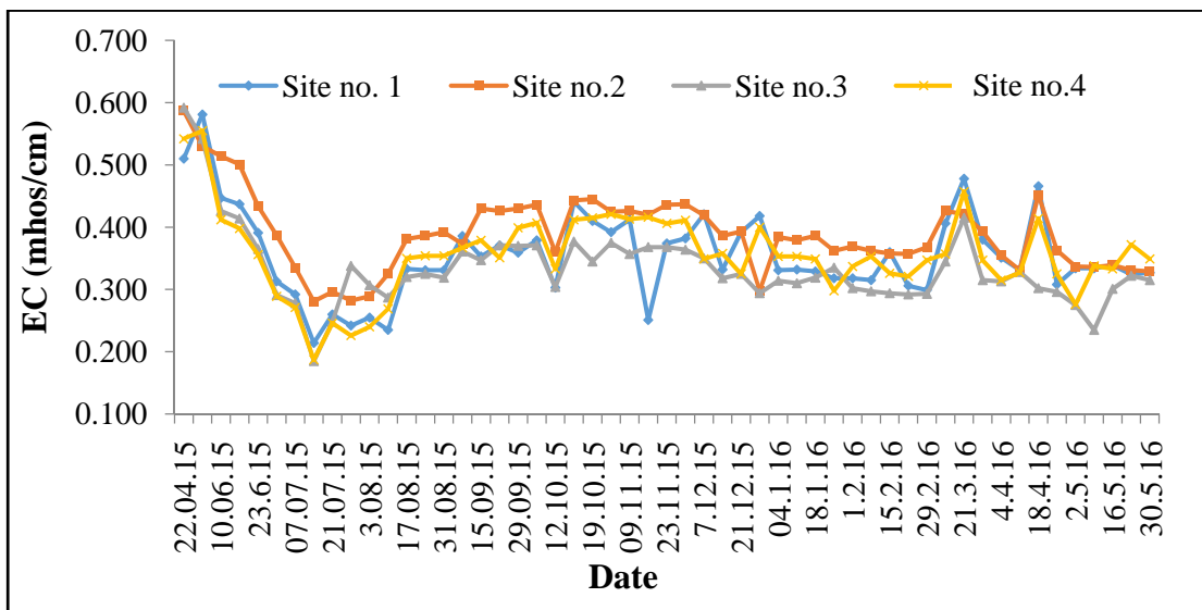
Fig. 4.6 Electrical conductivity (mhos/cm) values of groundwater samples at four sites
