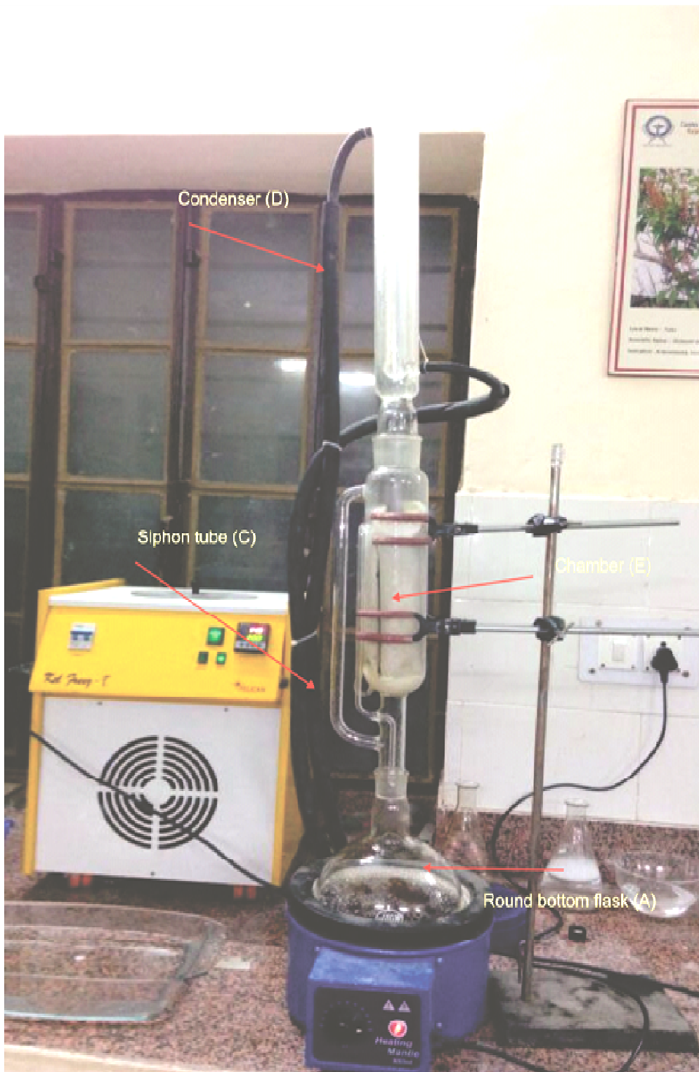
Figure 4: Photograph showing Extraction process by soxhlet method. (Soxhlet extraction assembly)
