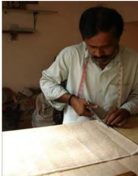
Plate 4. Bespoke method of cutting
