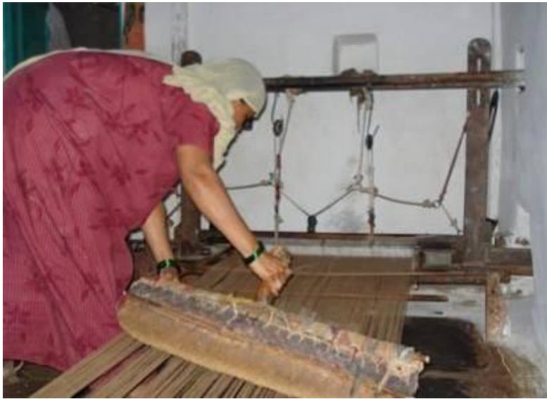
Brushing the warp sheet Plate 7. (contd...) Pre-loom processes
