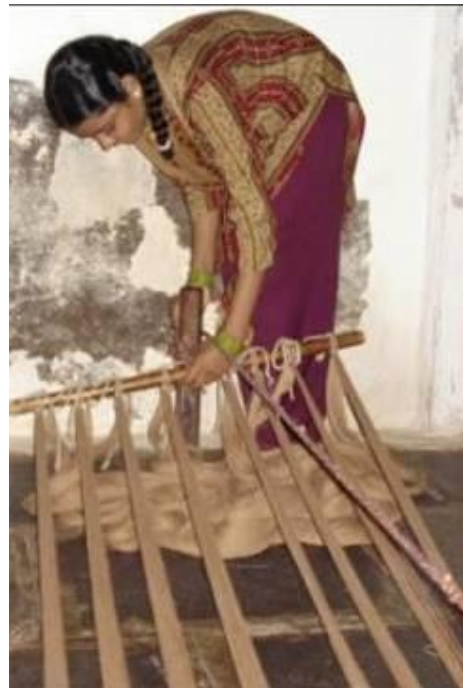
Tieing the other end of warp sheet to bamboo stave
