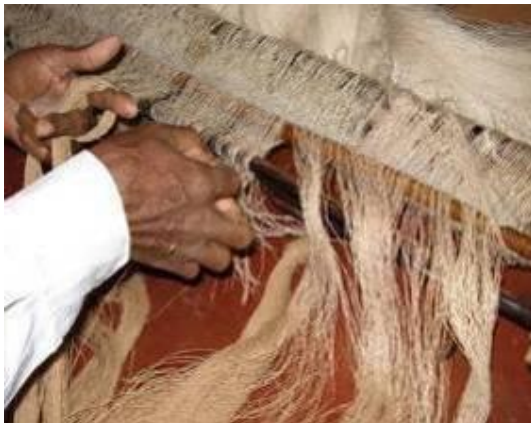
Twisting and joining the new Warp to previous warp ends
