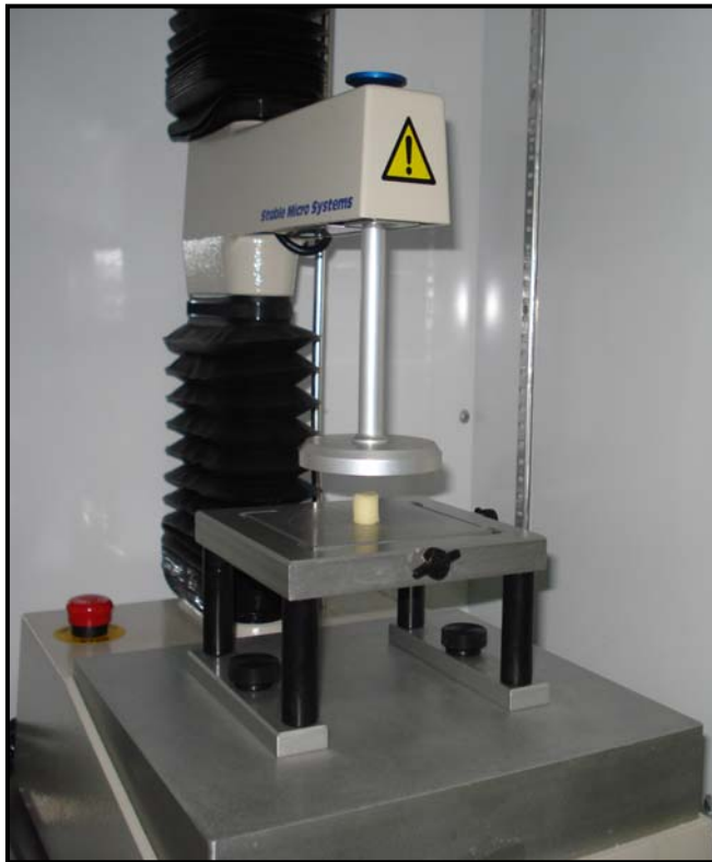
PLATE 3.4.2.3 a: Texture Profile Analyser with sample of danedar khoa
