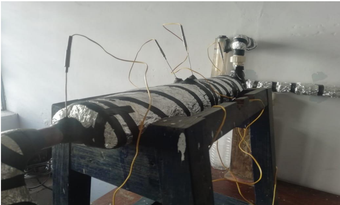
Fig 3.20 Thermal storage unit
