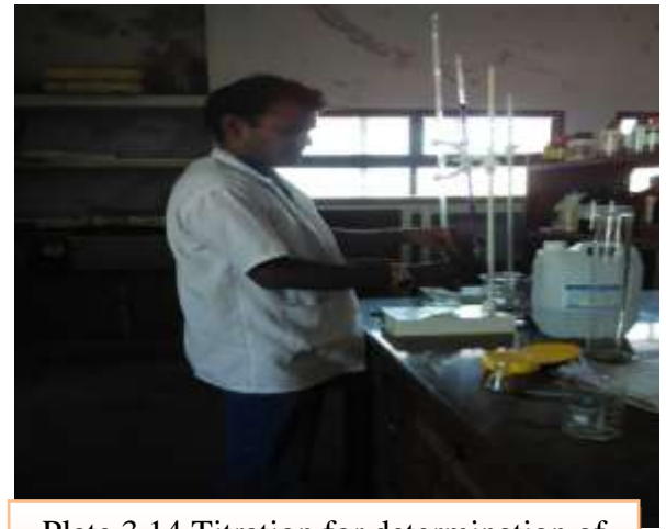
Plate 3.14 Titration for determination of acidity
