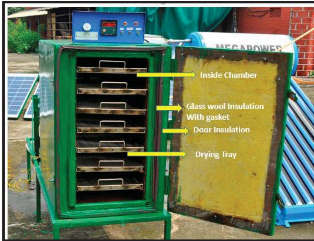
Plate 3.3. The fabricated dryer for vegetable seeds
