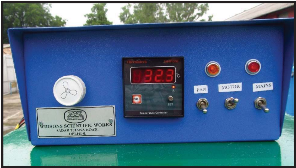
Plate 3.4. Temperature controller with fan speed control.
