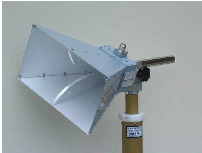
Fig. 1.18: Pyramidal microwave horn antenna, with a bandwidth of 0.8 to 18 GHz. A coaxial cable feedline attaches to the connector visible at top. This type is called a ridged horn; the curving fins visible inside the mouth of the horn increase the antenna's bandwidth (D.H. Werner, 2013)
