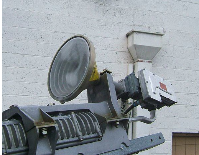
Fig. 1.19 : Corrugated conical horn antenna used as a feed horn on a Hughes Direcway home satellite dish. A transparent plastic sheet covers the horn mouth to keep out rain (D.H. Werner, 2013)
