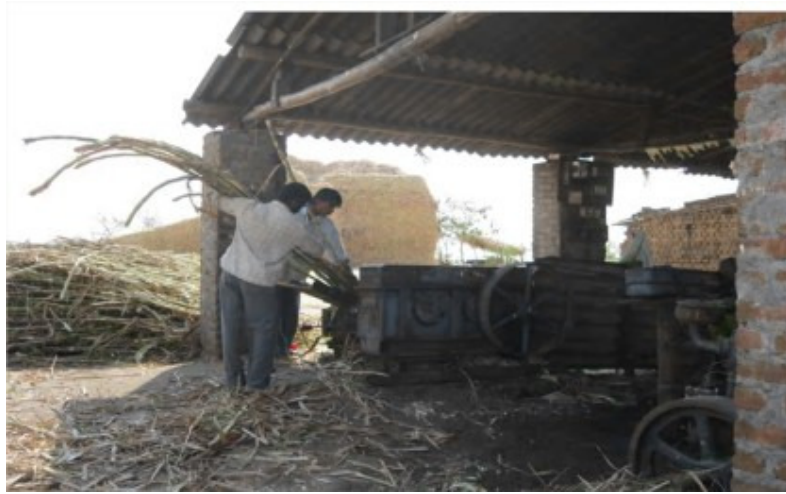
Manual feeding of sugarcane into juice extractor
