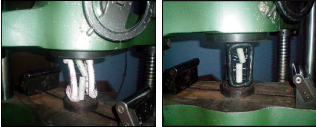
Fig. 8: Testing of ESF constructs under compression force using UTM.
