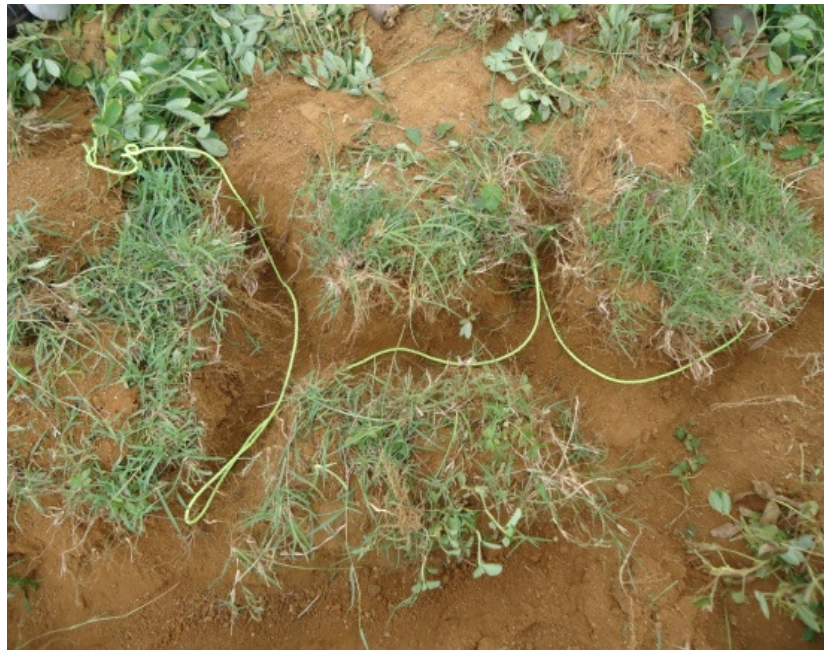
Plate 5. Excavated burrow on the bund
