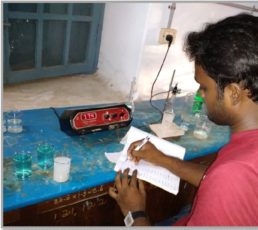
Plate 4.4: pH and EC analysis to test the chemical compatibility of insecticides and fungicides
