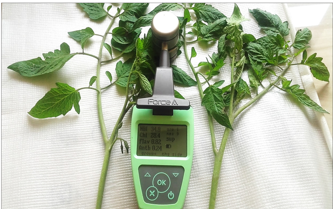
Plate 2b: DUALEX SCIENTIFIC+™ chlorophyll and polyphenol meter used for measuring total chlorophyll content, flavanol content and nitrogen balance index
