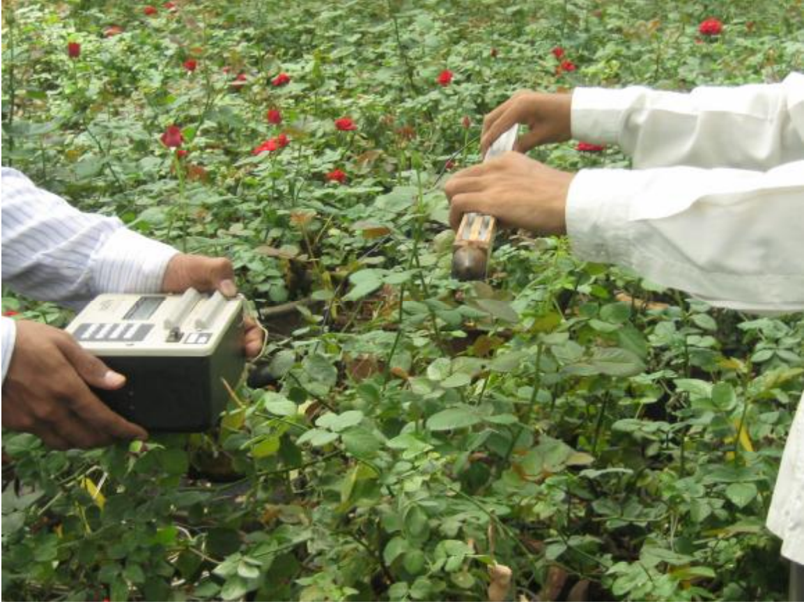
Plate No. - 2 Measurement of reflected radiation with the help of Line Quantum Sensor and Data Logger (LI-1000)
