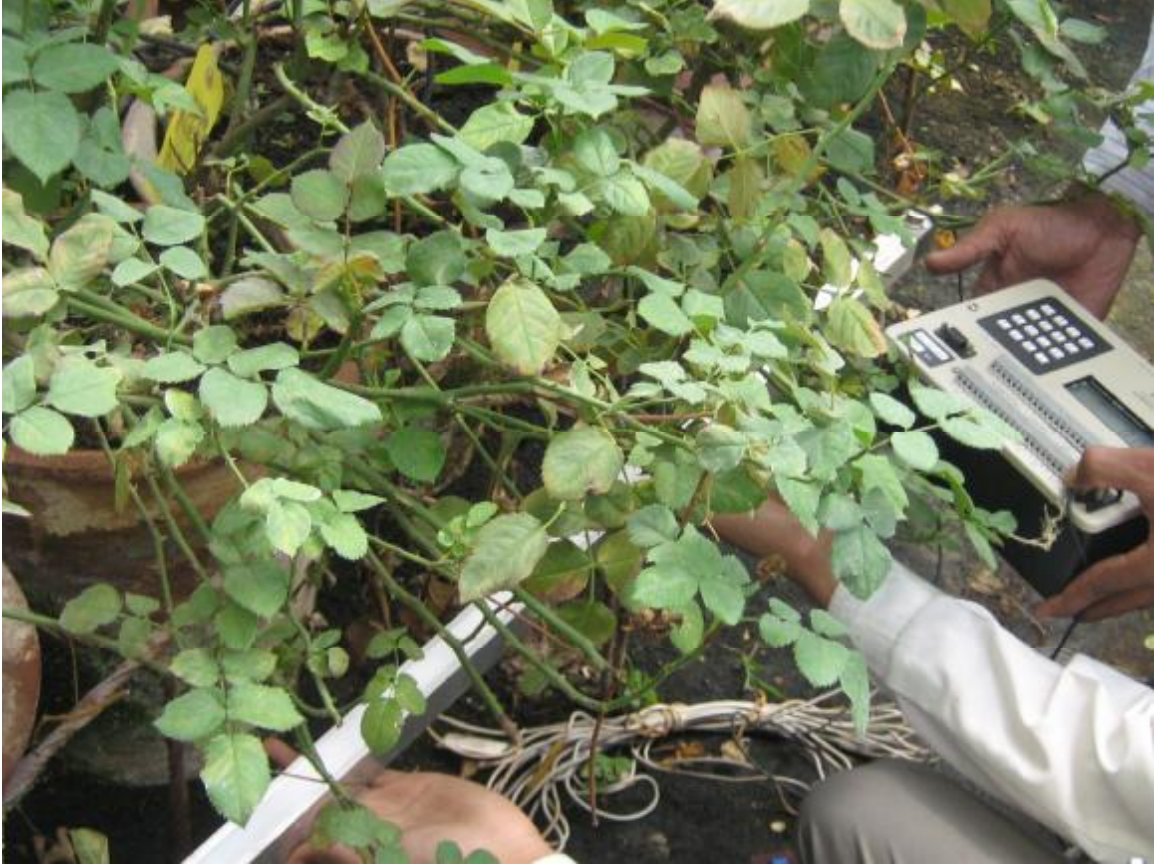
Plate No. - 3 Measurement of transmitted radiation with the help of Line Quantum Sensor and Data Logger (LI-1000)
