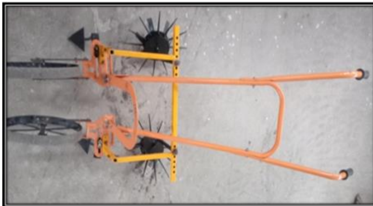
Fig. 3.14 Top view of developed finger weeder
