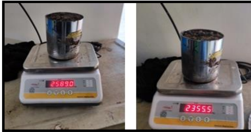
Fig. 3.17 Measurement of soil moisture content
