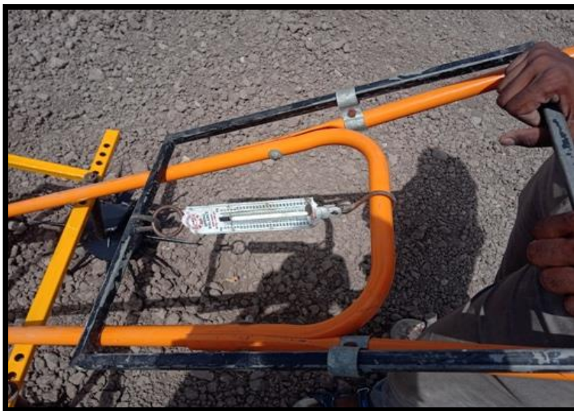
Fig 3.20 View of spring-type load indicator
