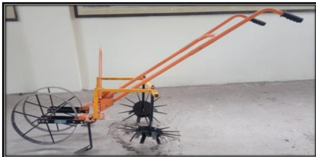
Fig. 3.16 Side view of developed finger weeder
