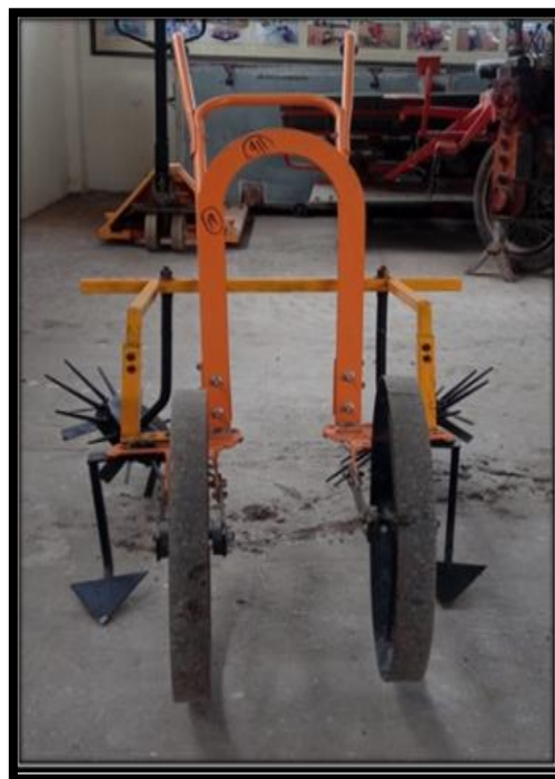
Fig. 3.15 Front view of developed finger weeder
