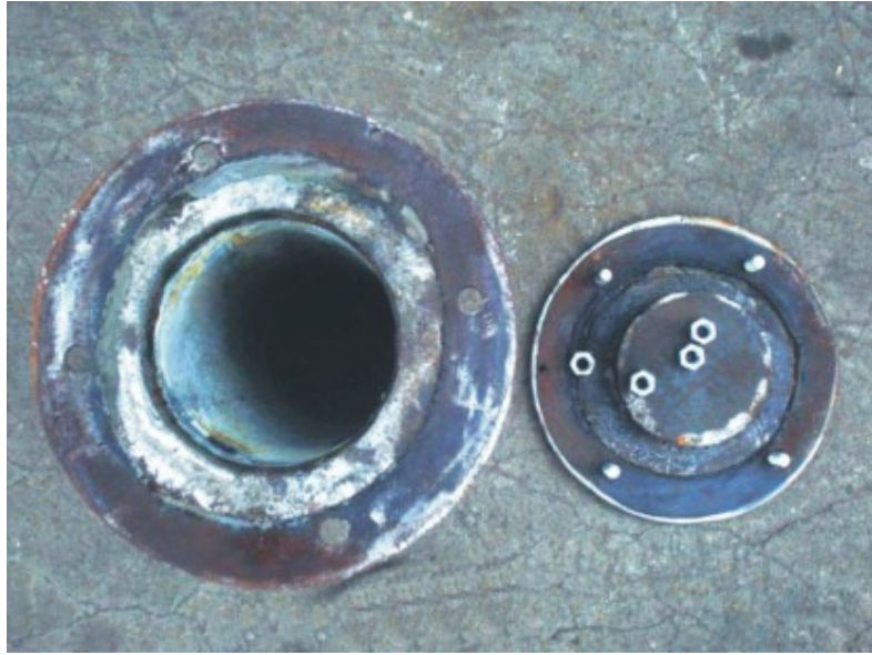
Plate 2a: Locally fabricated steel unit used for autohydrolysis of substrates
