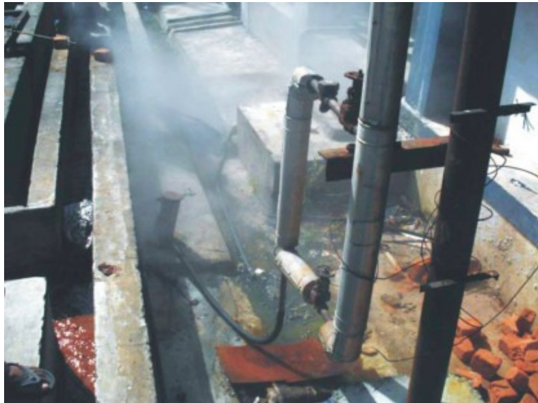
Plate 2b : Autohydrolysis of substrates with 200 0 C steam temperature at the S. L. N. Distillery, Garag
