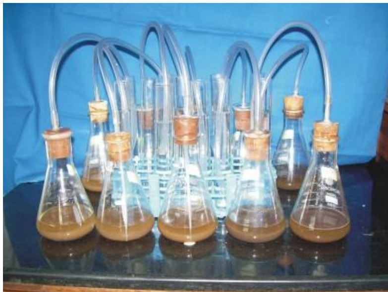
Plate 5b. Alcohol production using combined inoculations of Saccharomyces cerevisiae and Candida shehatae
