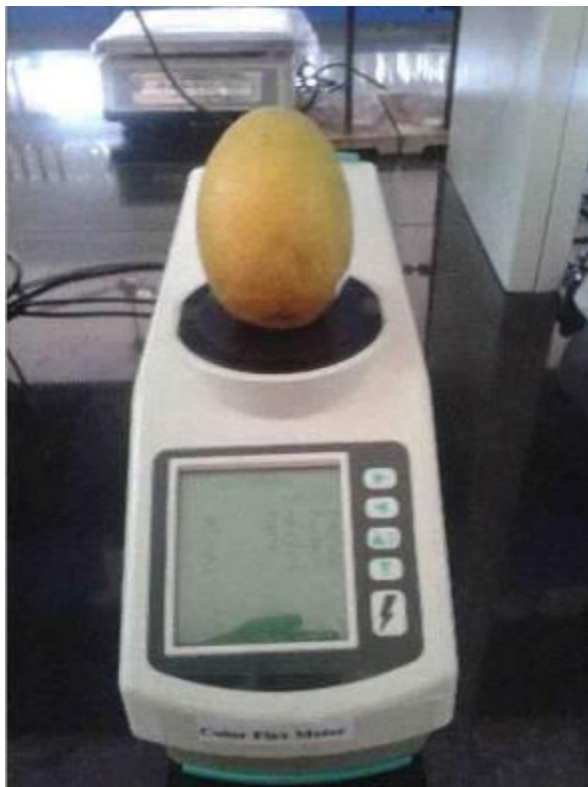
Plate 3: Measurement of fruits colour using Hunter Lab Colorimeter
