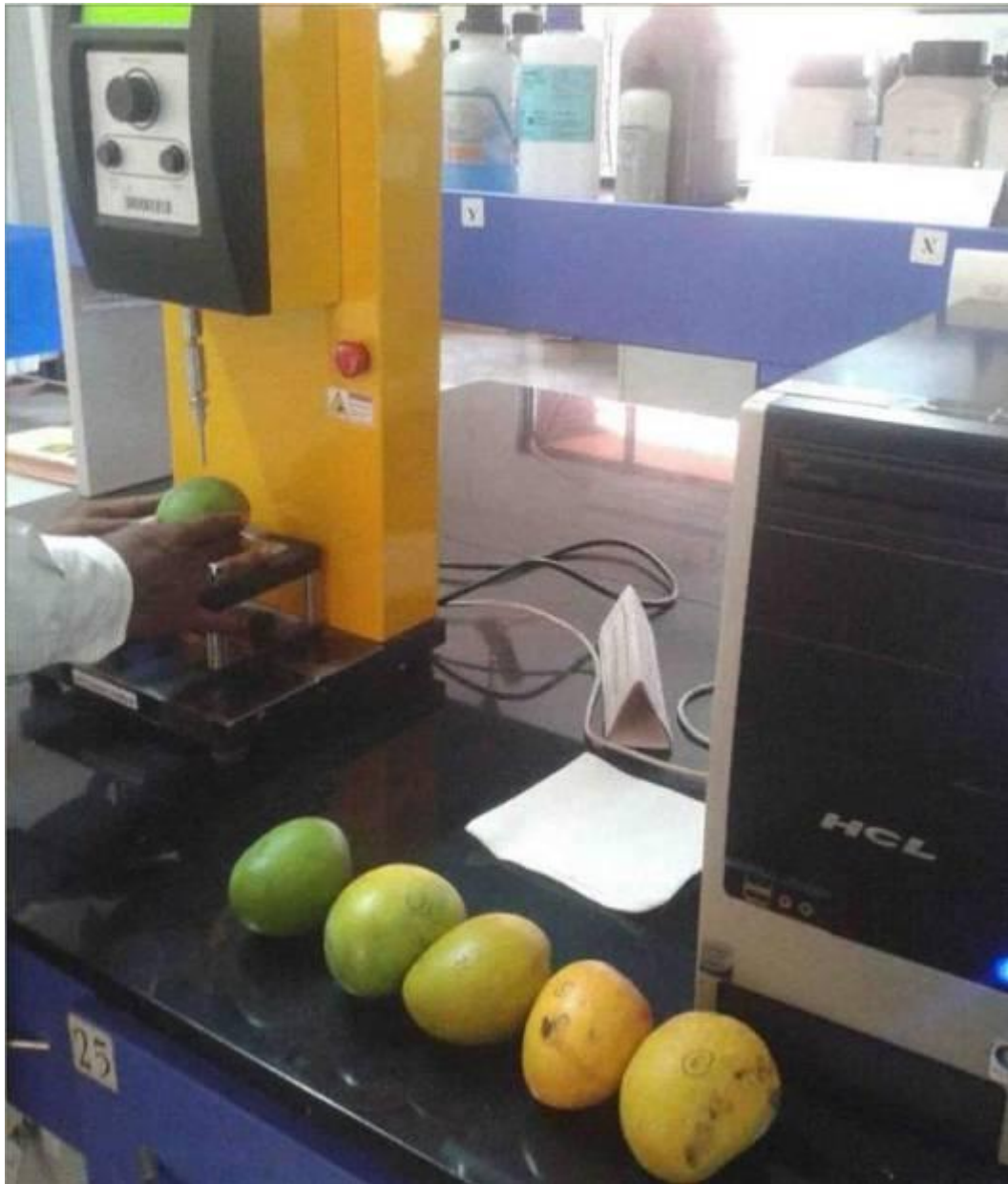
Plate 5 : Measurement of fruit texture using QTL Texture Analyser
