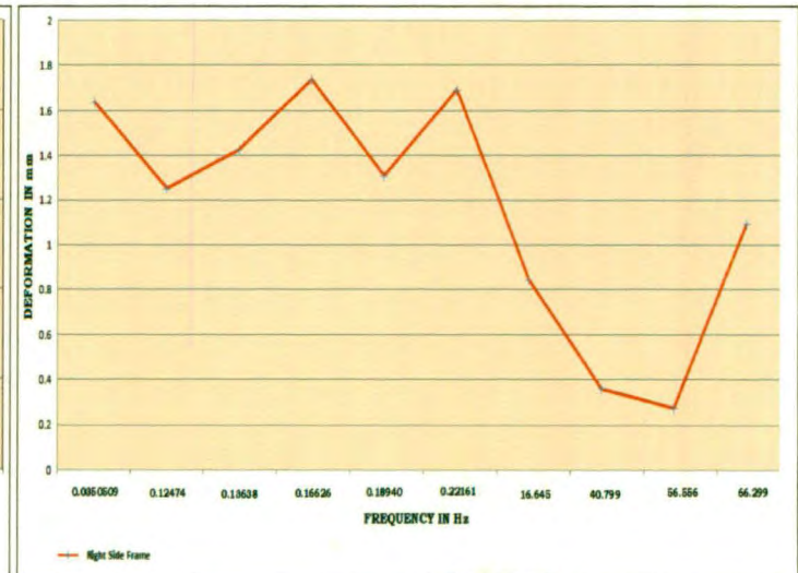
Deformation in right side frame
