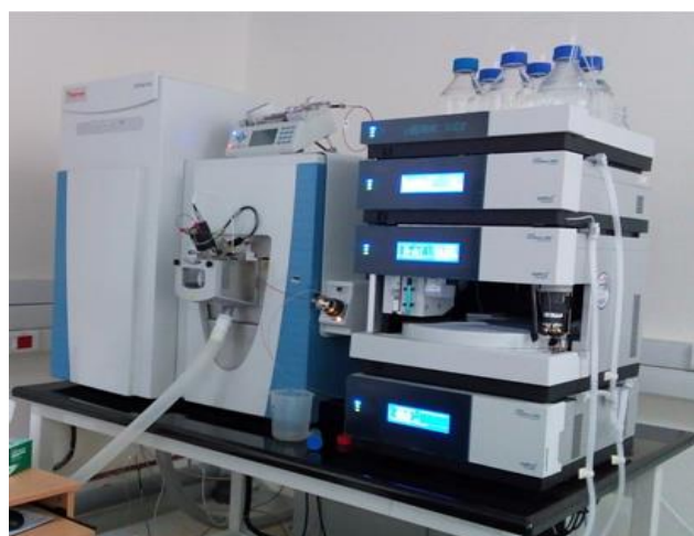
Fig.3.8. Thermo Scientific-Q ExactiveMass spectrometer coupled to a Thermo Scientific UltiMate 3000 UHPLC system
