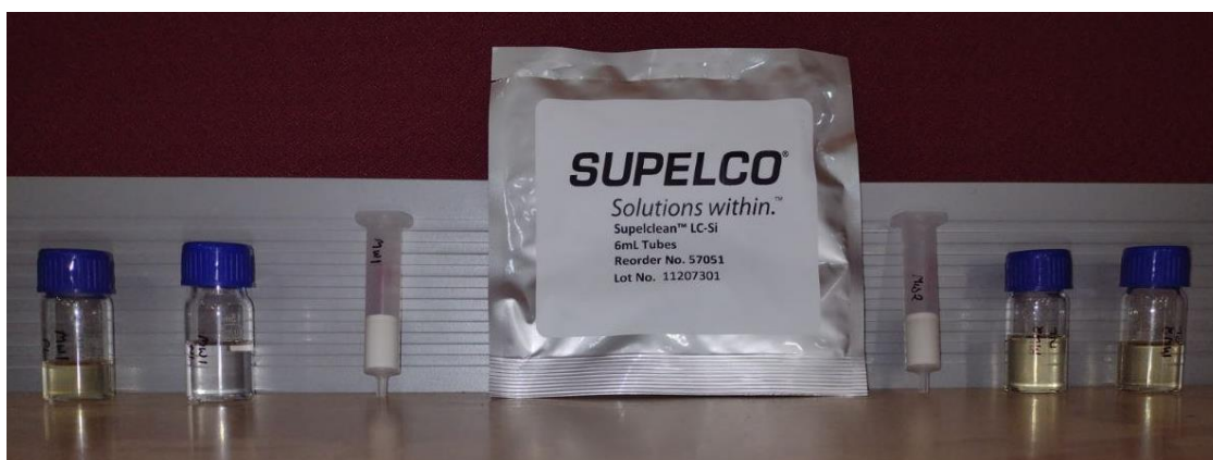
Fig. 3.3. Supelco disposable SPE tubes with eluted solvents in vials
