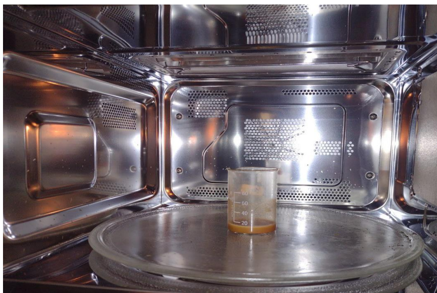
Fig. 3.11. Cavity of microwave unit with sample placed in beaker
