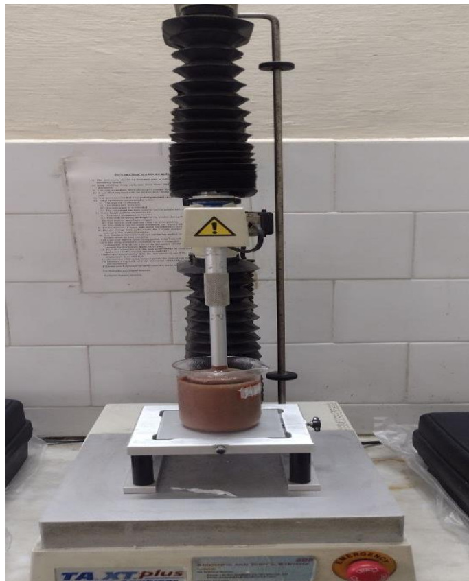
Fig. 3.6. Texture analyser used for texture profile analysis and back extrusion of ice cream
