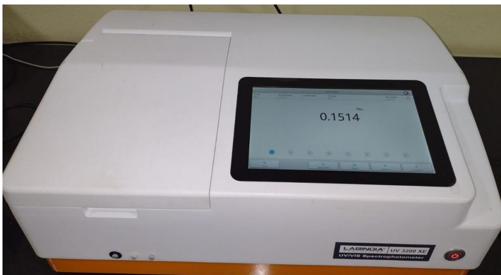
Fig 3.4. UV/VIS spectrophotometer (UV 3200 XE) used for measuring optical density
