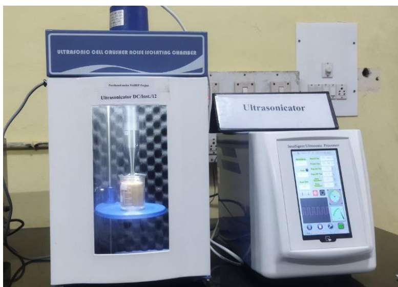
Fig. 3.12. Ultrasonication unit used for extraction of phospholipids from ghee residue
