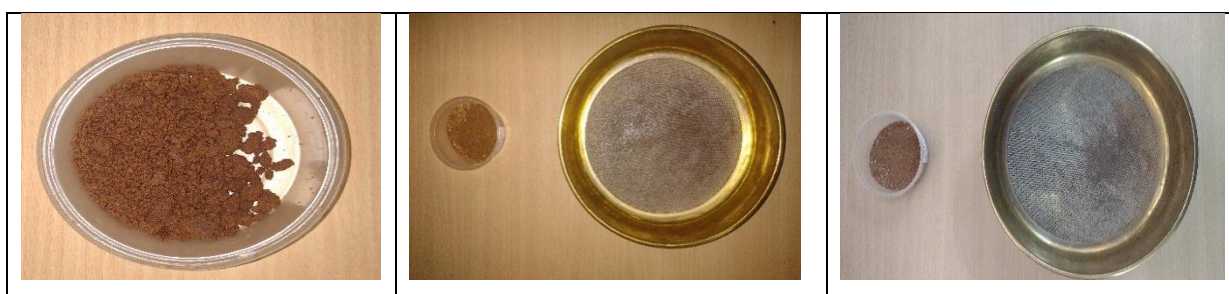
Fig.3.2. Ghee residue (a) after boiling water treatment; (b) particle passing through 0.25 mm sieve; (c) particle passing through 0.30 mm sieve
