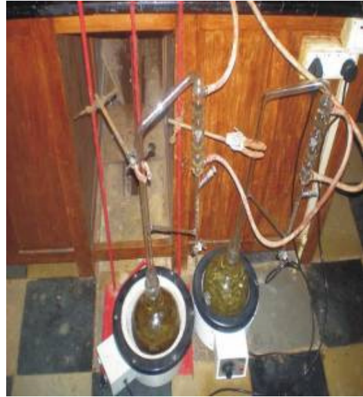
Clavenger-type oil extraction unit
