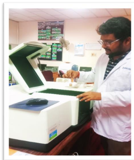
Fig. 3.9. Perkin Elmer Lambda 35 UV-Vis Spectrophotometer for the estimation of antioxidant status.
