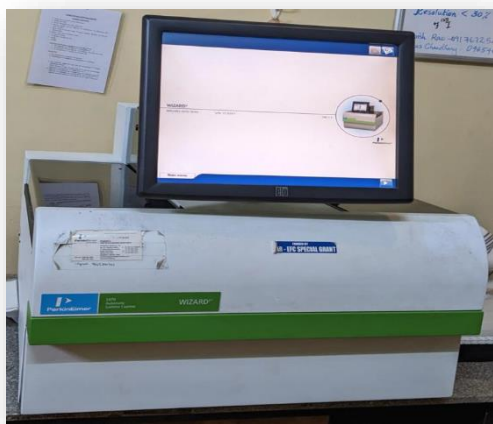
Fig. 3.7. Gamma counter for the estimation of serum cortisol by radio-immunoassay.
