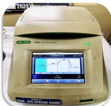
Fig. 3.12. Thermal cycler (Bio-Rad) for performing cDNA synthesis and gradient PCR.
