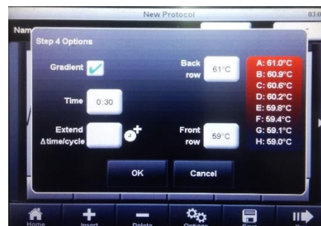
Fig. 3.12. Thermal cycler (Bio-Rad) for performing cDNA synthesis and gradient PCR.
