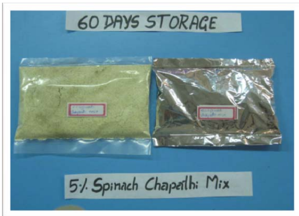
Plate 7 : Packaging materials used for storage of products (Low density polyethylene covers and laminated pouches)
